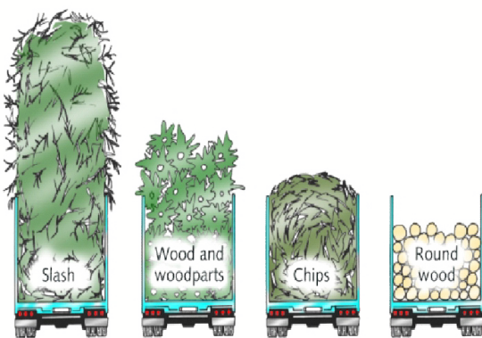
Figure 1. Energy Density Differences of the Same Weight Material by Different Product Types
